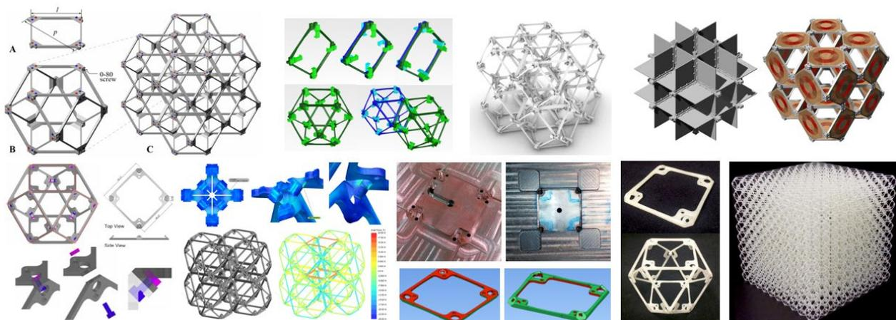
Figure 9: Discrete material system current work. Top (L to R) Cuboct voxel decomposition, robotically assembled latching design, plate lattice and EM discrete materials. Bottom (L to R) Low-cost Cuboct design, simulation of joints and beams, tooling and molding, part production, voxel assembly, and 10x10x10 cube.
