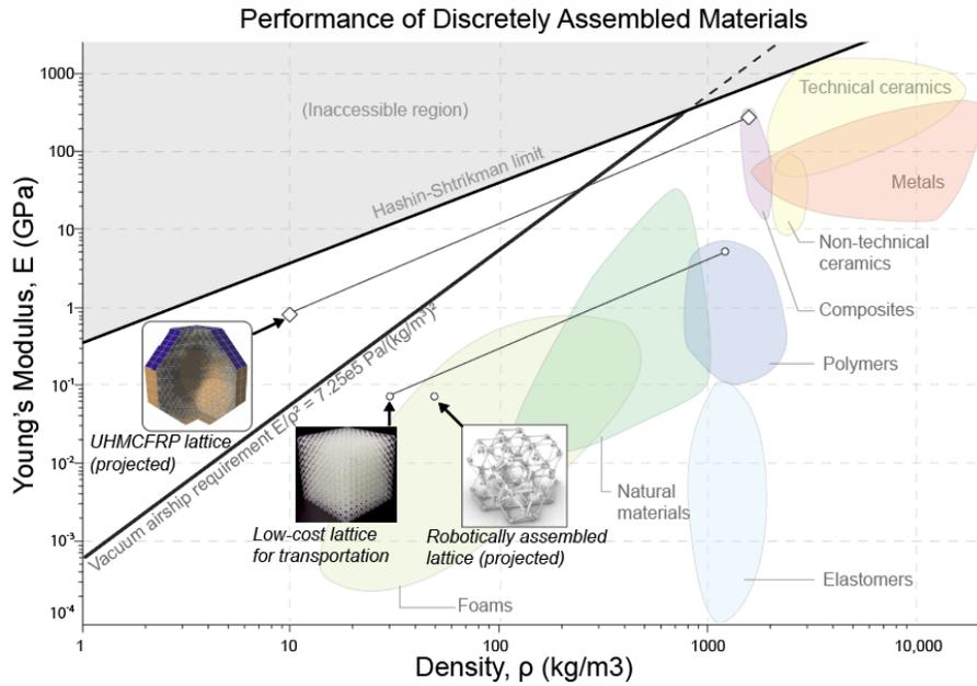
Figure 14: Projected discrete material properties for robotic assembly, low-cost transportation, and LTA buoyancy. Objectives include accessing novel material property space and defining performance of robotically assembled materials.
