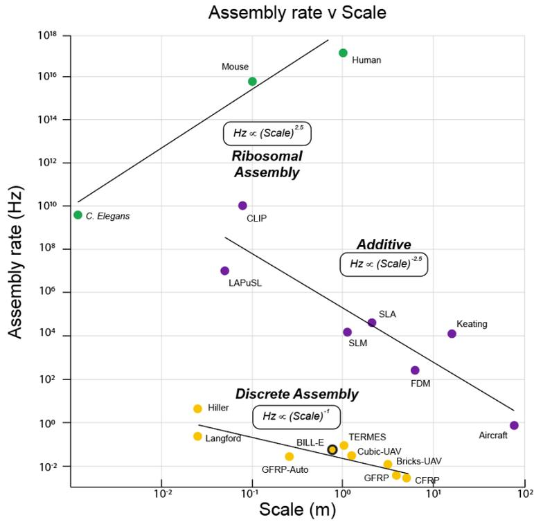
Figure 16: Assembly rate v Scale. The positive slope of biological growth is attributable to recursion. While this thesis will not address recursion, I will demonstrate increased scale and throughput through parallelization.
