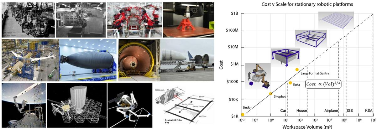
Figure 3: Automation and digital fabrication. Machines scale with the size of the part, with associated cost increase.
