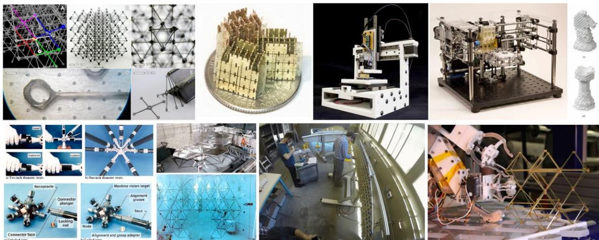
Figure 5: Discrete materials and assembly. Planar lattice elements [30], electronic bricks [31] and spherical voxels [32], with gantry-style assembly platforms. Robotic and manual assembly of strut-and-node systems [36] and voxels [37][38].
