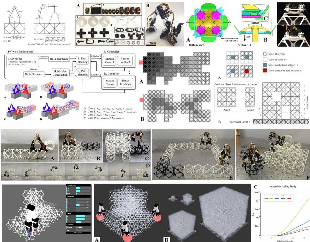
Figure 11: Relative Robotics current work. System Design (Row 1, L to R): Kinematics, actuation, end effectors, sensing. Control Strategies (Row 2, L to R): Centralized architecture, build sequence, coordination, path planning. Assembly testing (Row 3, L to R): 1D, 2D, and 3D construction, global precision using local metrology, multi-robot construction. Software environment (Row 4, L to R): single robot control and motor outputs, multi-robot simulation, large scale simulation and evaluation.
