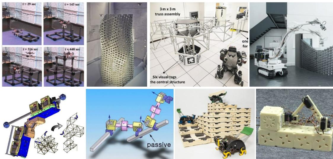
Figure 6: Mobile robotic assembly systems. UAV truss [45] and brick [43] assembly, wheeled robot truss [46] and brick [44] assembly, structure-traversing truss [47][48] and brick robots [41][42].
