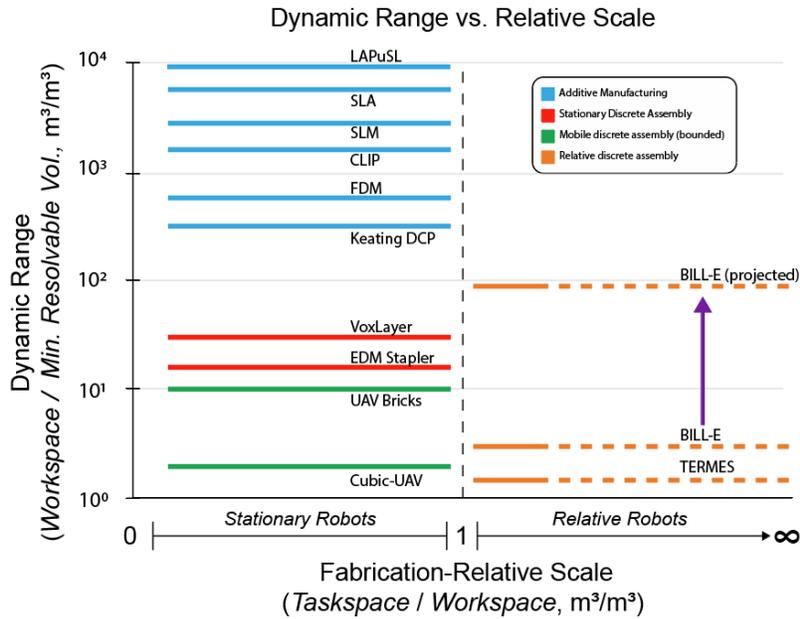
Figure 17: Stationary platforms have large dynamic range, but limited workspace. Relative robots can occupy an unoccupied part of parameter space for robotic fabrication.
