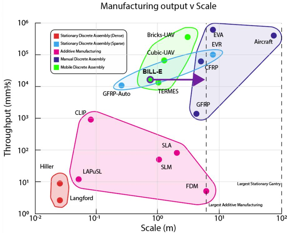
Figure 15: Current and projected robotic throughput and scale, with direction of projected performance indicated. The goal is to maintain high volumetric throughput at larger scales to compete with state of the art assembly.
